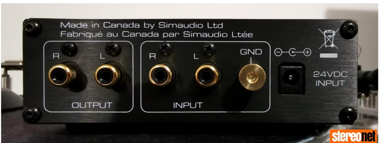
Around the rear, you'll find two output and two input RCA jacks, and a ground post, all of which are gold-plated. There's also the input jack for the 24V power supply which remains on at all times. Don't worry though; this thing sips at the juice. Even the wall wart power supply looks better than average with its fabric-covered cord.
