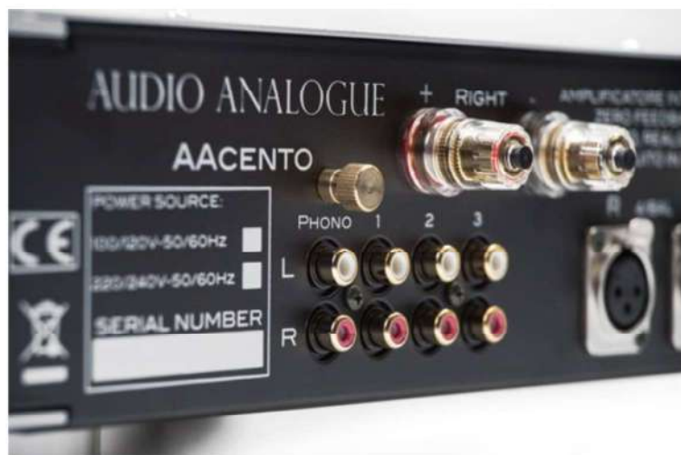
Although there is only one phono input, it can be switched to accommodate either moving-magnet (MM) or moving-coil (MC) cartridges.
