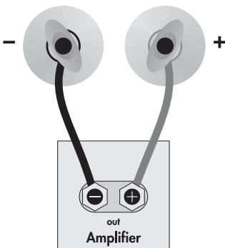
**Fig. 1b:** Single-wire connection.
