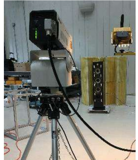
FIGURE 7 – LASERVIBROMETER TESTING AT THE NRC.
