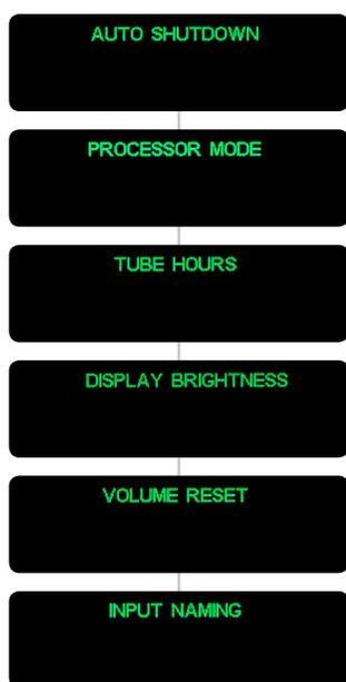
While a menu item is displayed, press 'ENTER', followed by rotating the volume knob on the front panel, or using the volume up/down buttons on the remote to adjust the settings of that particular selection. After making the appropriate change, pressing the 'ENTER' button will confirm the new setting, and the display will show 'OKAY' for five seconds before reverting back to the normal operation screen.
